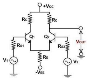
ground. In other words, there is some dc voltage at the output terminal without any input signal applied. DC analysis is exactly same as that of first case.
