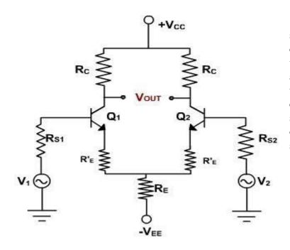
By using external resistors R'E in series with each emitter, the dependence of voltage gain on variations of r'e can be reduced. It also increases the linearity range of the differential amplifier shows the differential amplifier with swamping resistor R'E. The value of R'<sub>E</sub> is usually large enough to swamp the effect of  $r'_{E}$ .
